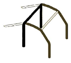
Two lateral rollbars two transversal members two backstays six mounting feet With this construction the diagonal member must be made double as a cross, right behind the seats.
