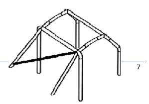
The cage must have one of the diagonal members shown on following drawing. The orientation of the diagonal member be reversed, and made double as a cross. Members must be straight. Diagonal member may also be mounted in the Bbar. Diagonal member may also be designed as an inverted V, but then must also the roof reinforcement be shaped like a V.
