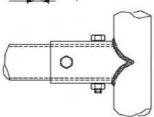
The removable connections type 1 (left) and 2 (left under & under) must be used for joining the upper parts of the main rollbar, the front rollbar and the lateral half-rollbars together.
