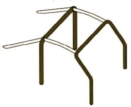
One B-bar Two lateral half-rollbars one transversal member two backstays six mounting feet
